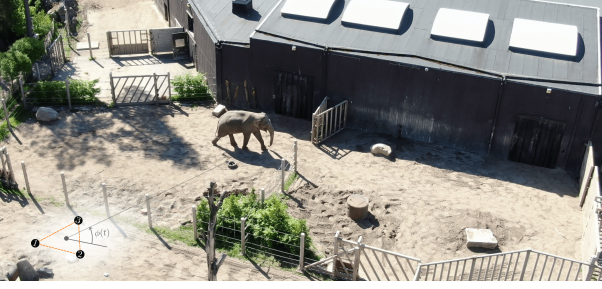
Fig. 5: The setup of the geophone network at Kolmården. The DOA angle is denoted \phi(t) . The elephant walks in front of the geophone network at a distance of 8–30 m.
